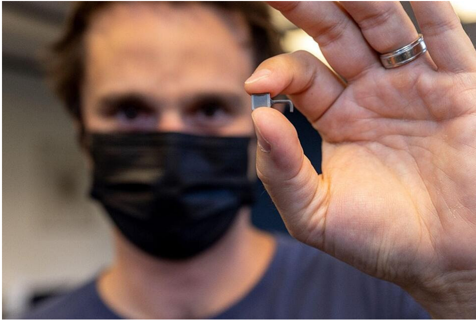
Paradromics' BCI consists of over 1,600 Platinum-iridium microwires
